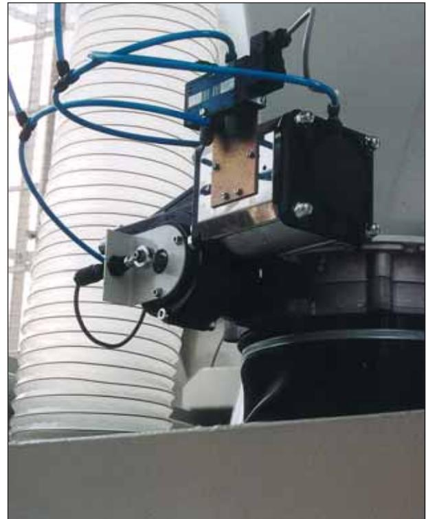
*Upon request, the mixer can be fitted with intake connection for additives and an air-bleed hose to be connected to the cement scale and filter.*
